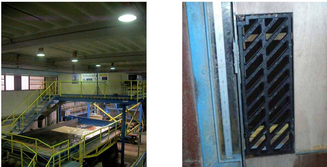
**Figure 1:** Physical model. Flume facilities (left) and inlet “Barcelona1” (right). Source: [11].
